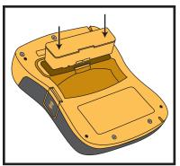
Before inserting the battery pack into the DDU-2000 Series AED as shown at left, ensure that the battery pack opening in the back of the AED is clean and clear of any
