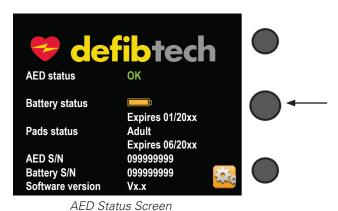
To check the status of the AED when the unit is off, press the **center softkey button**. The display screen will show unit status, battery pack status, and pad status. After a short period of time, the display screen, and the unit will turn off.
