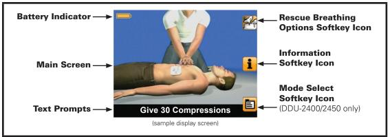
Battery Indicator - The Battery Indicator indicates the approximate remaining battery capacity.
