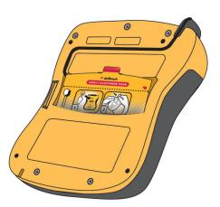
**STEP 1:** *Inspect the Pads* – First, check to ensure that the pads package has not expired (see diagram in Section 3.2). Do not use pads past their expiration date. Discard expired pads. Next, check to ensure that the pads package has not been torn, opened, or damaged. Dispose of the pads if the package is open or damaged. Inspect the pads cable and replace pads if any nicks, cuts, or broken cables are found.
